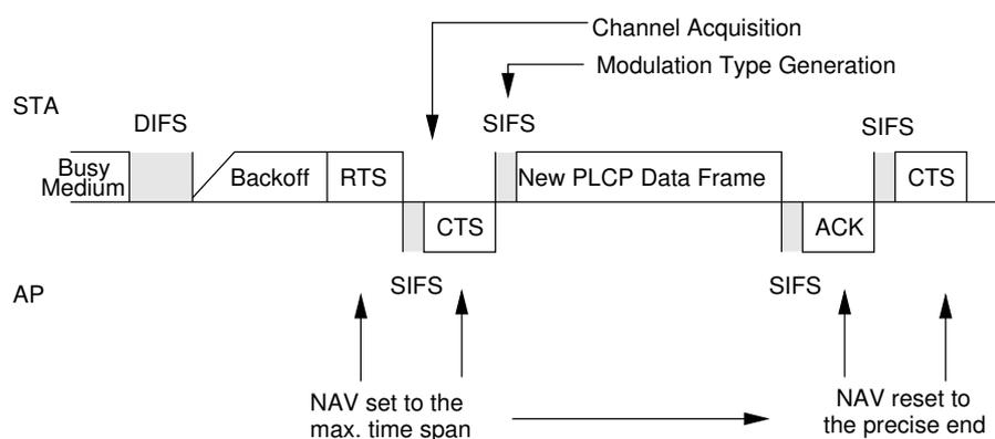
Figure 3.1: Transmission sequence of the new concept. In order to set the NAV correctly, a slightly modified transmission sequence is required.
