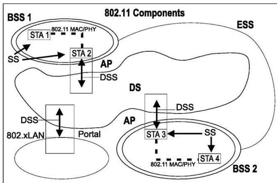
Figure 2.1: 802.11 architecture of the infrastructure mode.
