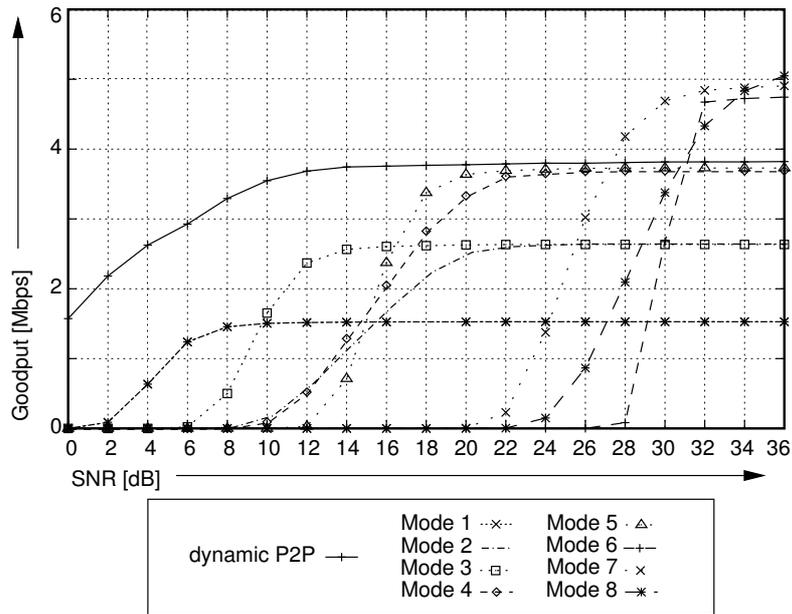
Figure 3.8: Performance comparison of 802.11 DYN and legacy IEEE 802.11a with RTS/CTS for various different SNR levels for a packet size of 228 Byte.
