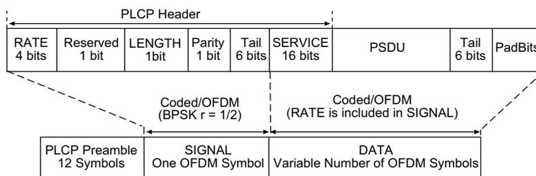
Figure 2.6: 802.11 OFDM PPDU frame format
