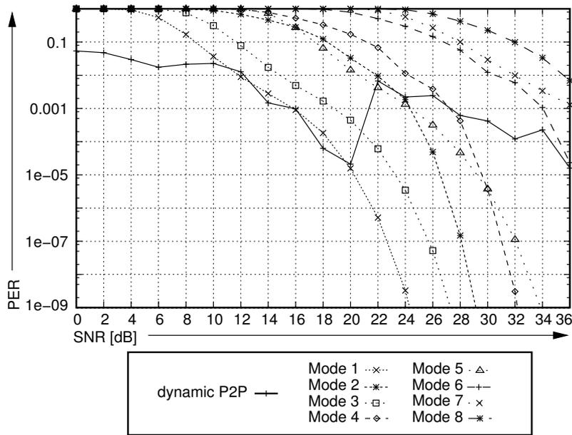
Figure 3.10: Comparison of the packet error rate for all legacy 802.11a modes and 802.11 DYN with adaptive modulation (regarding a packet size of 228 Byte and a varying SNR).
