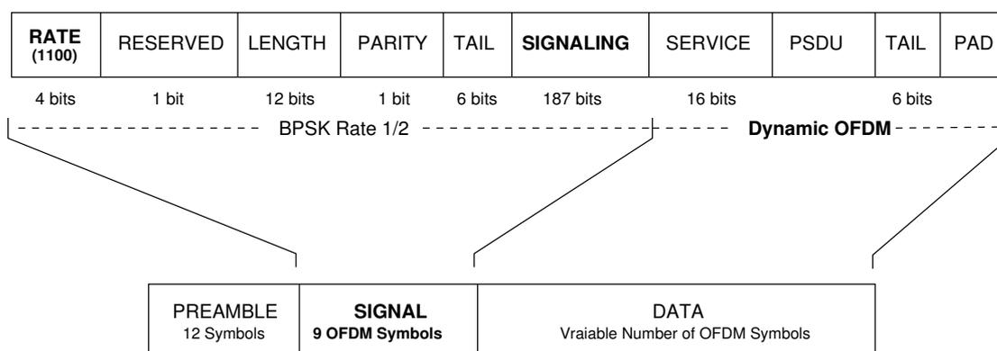
Figure 3.2: Structure of the new PLCP frame.
