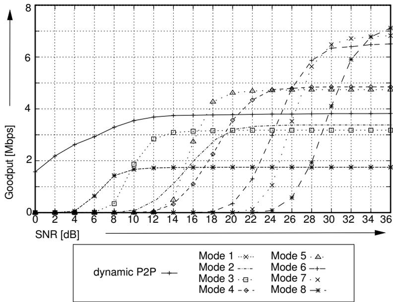
Figure 3.9: Performance comparison of 802.11 DYN and legacy IEEE 802.11a without RTS/CTS for various different SNR levels for a packet size of 228 Byte.
