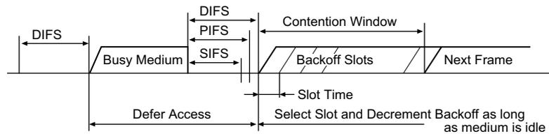
Figure 2.2: DCF-based medium access
