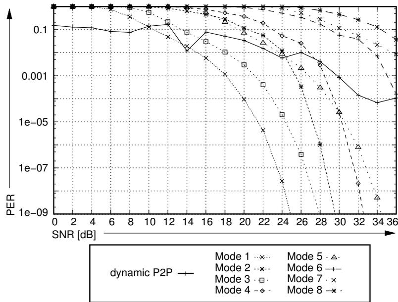
Figure 3.6: Comparison of the packet error rate for all legacy 802.11a modes and 802.11 DYN with adaptive modulation (regarding a packet size of 1564 Byte and a varying SNR).
