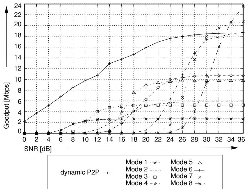
Figure 3.5: Performance comparison of 802.11 DYN and legacy IEEE 802.11a without RTS/CTS for various different SNR levels for a packet size of 1564 Byte.
