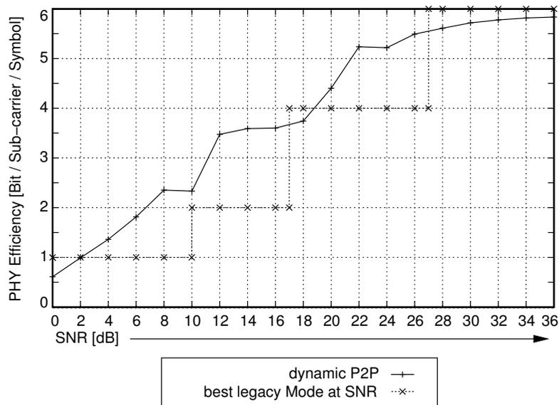
Figure 3.11: PHY efficiency (in terms of bit per sub-carrier per symbol) for 802.11 DYN and legacy IEEE 802.11a in case of a packet size of 228 Byte.
