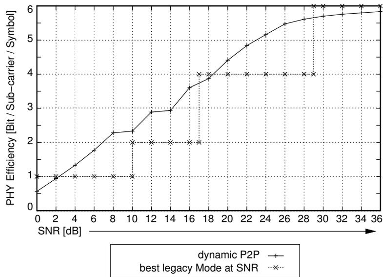
Figure 3.7: PHY efficiency (in terms of bit per sub-carrier per symbol) for 802.11 DYN and legacy IEEE 802.11a in case of a packet size of 1536 Byte.
