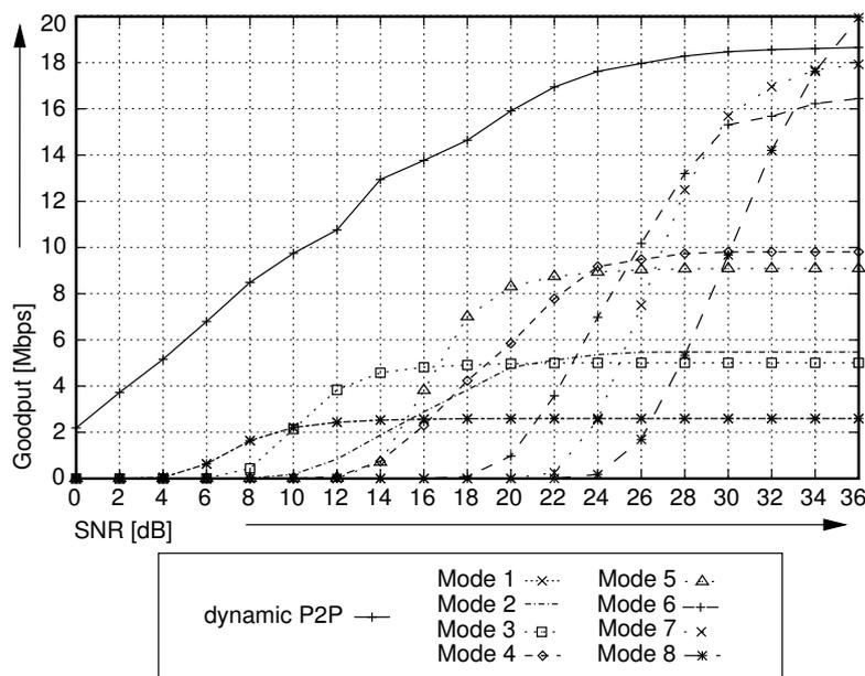
Figure 3.4: Performance comparison of 802.11 DYN and legacy IEEE 802.11a with RTS/CTS for various different SNR levels for a packet size of 1564 Byte.
