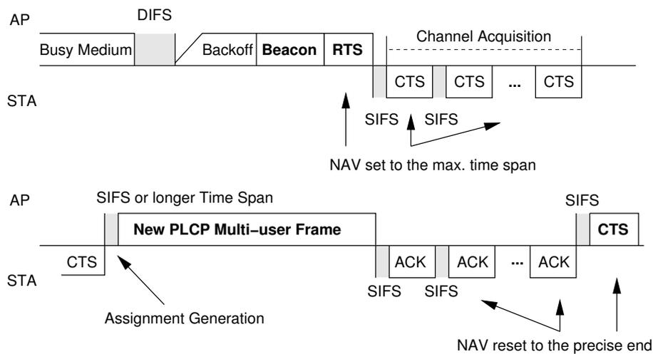
Figure 4.1: Transmission sequence of the new concept in the case of the point-to-multi-point communication mode (down-link, i.e. access point to stations).
