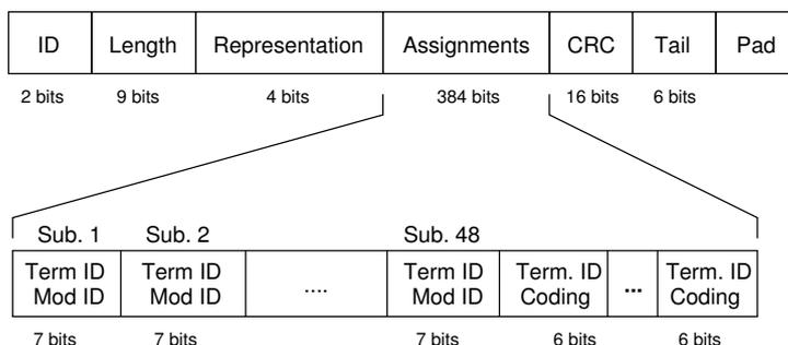
Figure 4.2: Structure of the Signaling field in the point-to-multi-point communication mode (down-link, i.e. access point to stations).
