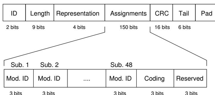
Figure 3.3: Structure of the new Signaling field.
