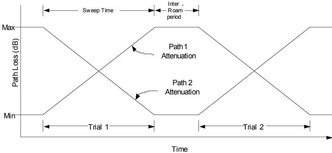
Fig. 2.4 Path loss profiles to be produced by the variable attenuators shown in Fig. 2.1
