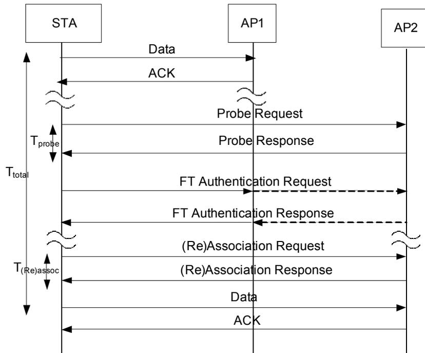
Fig. 3.3 Fast BSS Transition with Authentication Exchange over the DS
