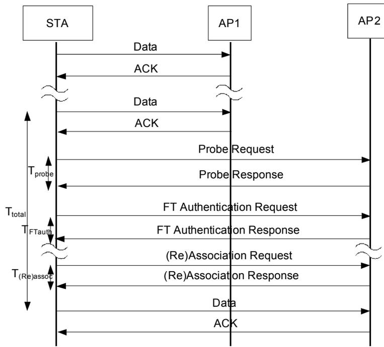
Fig. 3.2 Fast BSS Transition with Authentication Exchange over the air
