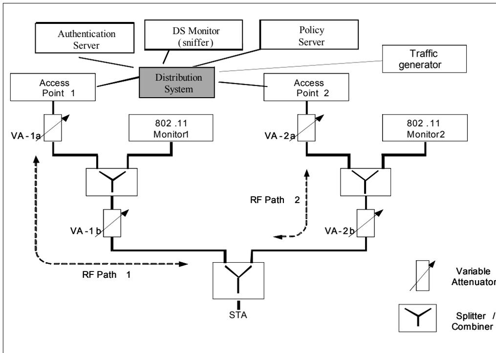
Fig. 3.1 Fast BSS Transition Test Set-up
