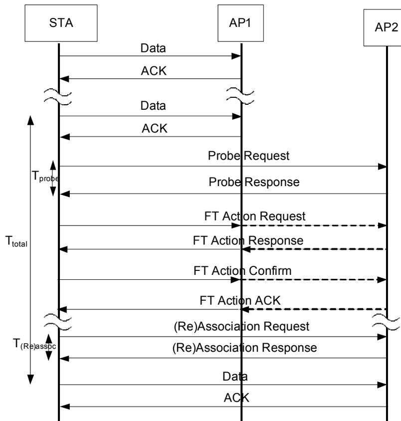
Fig. 3.5 Fast BSS Transition with Pre-Reservation Over the DS (And Auth Exchange over the DS)
