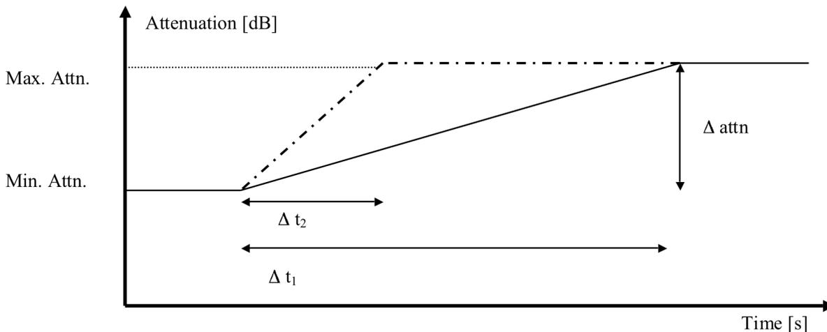
Fig. 2.2: Linear attenuation change (sweep function linear in dB) through one path
