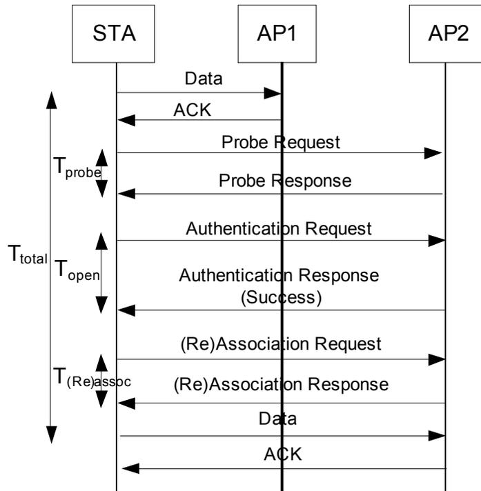
Figure 2.3 Open System Authentication
