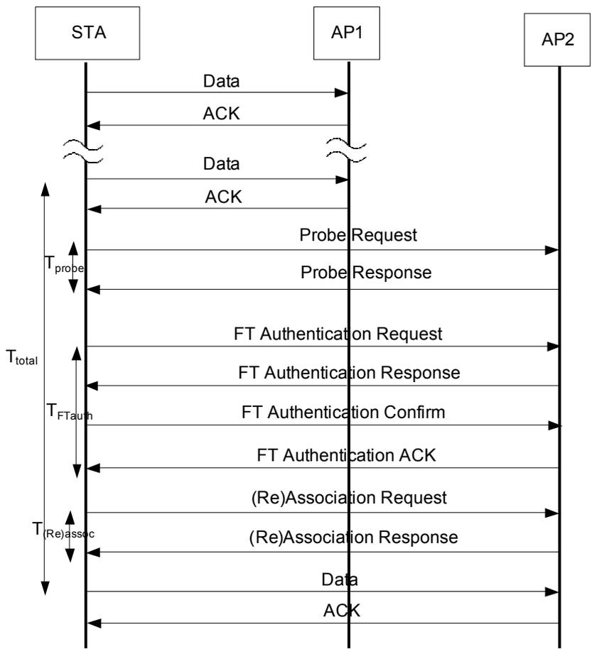
Fig. 3.4 Fast BSS Transition with Pre-Reservation Over the Air (And Auth Exchange over the Air)
