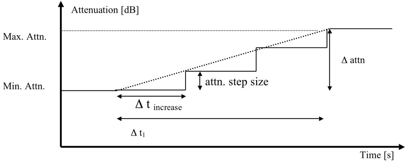
Fig. 2.3: Stepwise increase of imposed attenuation
