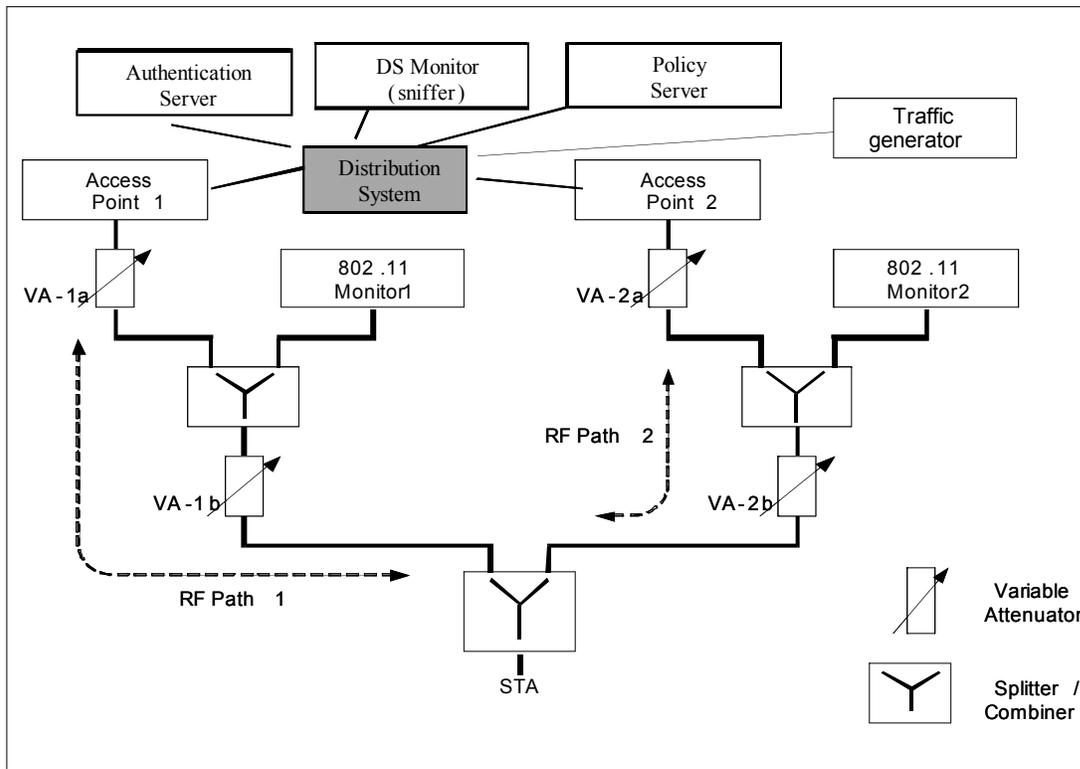
Fig. 2.1 BSS Transition measurement Test Set-up
