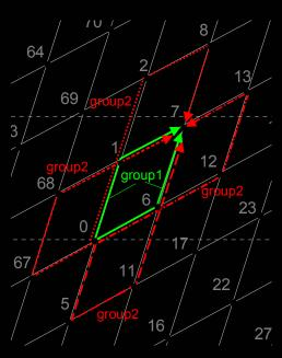
Clear path group separation by cost ranges (costs = accumulated propag. + processing delays)
